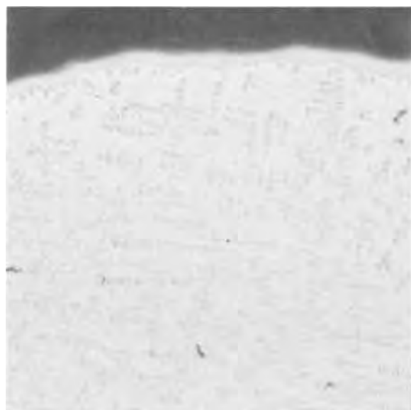
Fig. 4. Photomicrograph of a typical ThN scale growth that was formed on liquid thorium in 1520 Torr nitrogen at 2100°C (X100).
