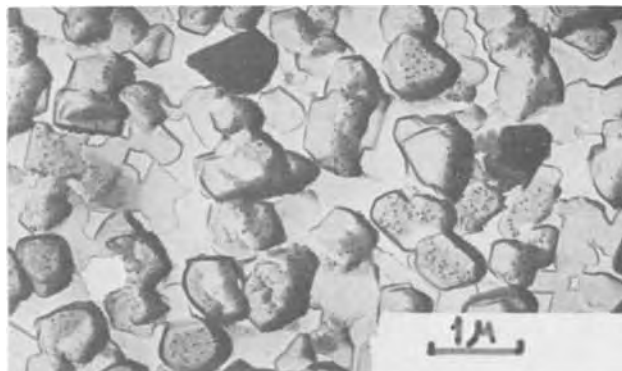
Fig. 1 (b). Platinum-carbon replica of the surface of V 2 O 3 deposited onto mica. Particles of V 2 O 3 are partially extracted. Shade angle is 10°.
