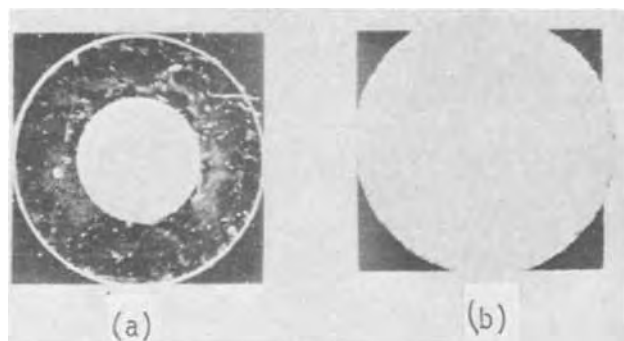
Fig. 2. Bottom view of electrostatically sealed piezoresistive pressure transducers. (a) Borosilicate glass cavity, (b) Silicon cavity.
