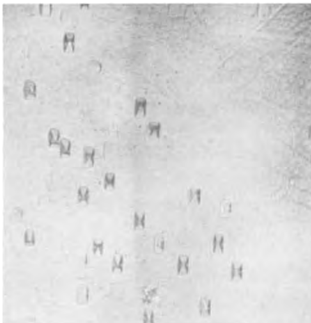
Fig. 1. Dislocation etch pits produced on the (001) face by dilute HNO 3 (40%), \times 400 .
