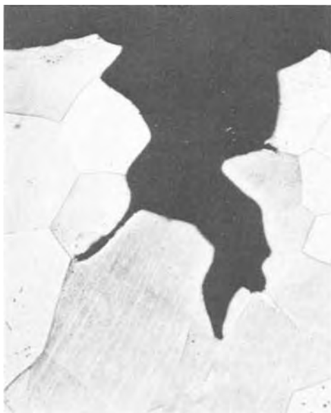
Fig. 6. Stress corrosion cracking in water-quenched 18% chromium, 1.5% nickel stainless steel, MgCl_2 , 130^\circ C , showing both transgranular and intergranular cracks. Magnification X90.
