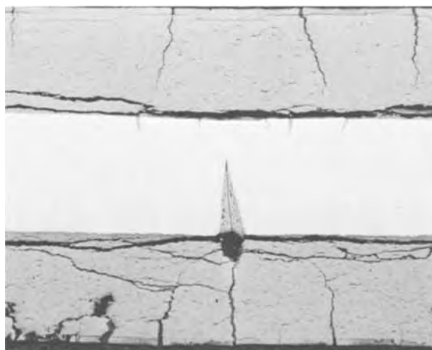
Fig. 3. Oxide wedges formed in niobium tensile specimens oxidized at 435°C in air while a constant tensile stress of approximately 15,000 psi was applied; 100X.
