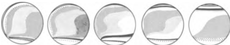
Fig. 3. Silicon wafers with nonuniform thickness of silicon nitride.
