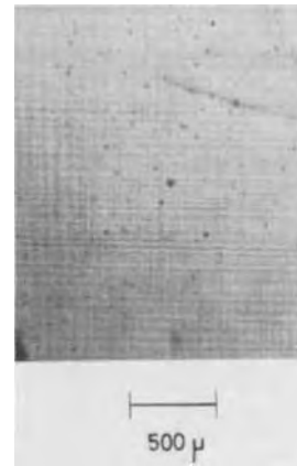
Fig. 3. The optical photograph of the surface which reveals the cross-hatch pattern.
