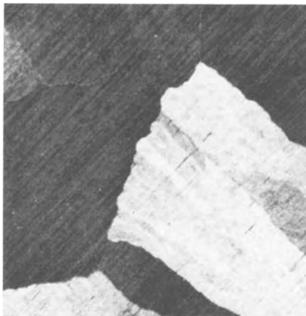
Fig. 1. Hard aluminum foil given a 5 min dip in boiling water prior to a 550°C anneal in air; oblique illumination. (X10).
