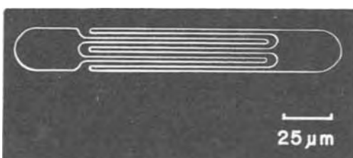
Fig. 6. Dark-field light micrograph of interdigitated 2.5 \mu\text{m} lines etched in 4000\text{\AA} of \text{SiO}_2 .
