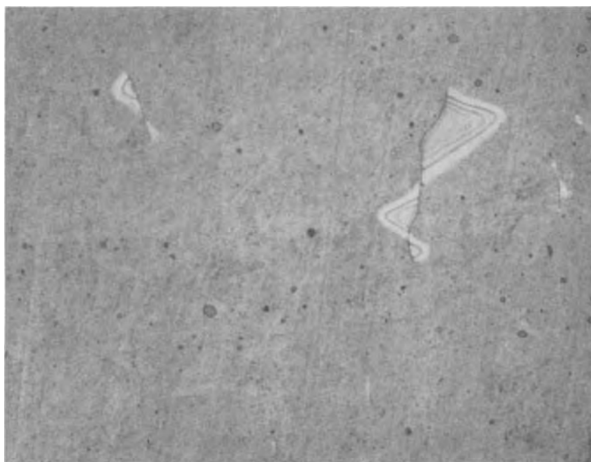
Fig. 7. Photomicrograph of silicon nitride-coated copper strained 1% in tension. Cracks are readily identified by interference fringes adjoining crack.
