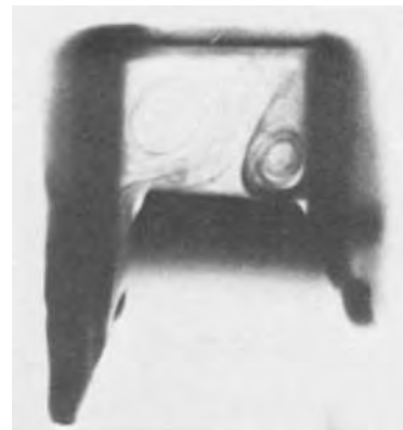
Fig. 2. Vortex patterns produced in a rectangular tube
