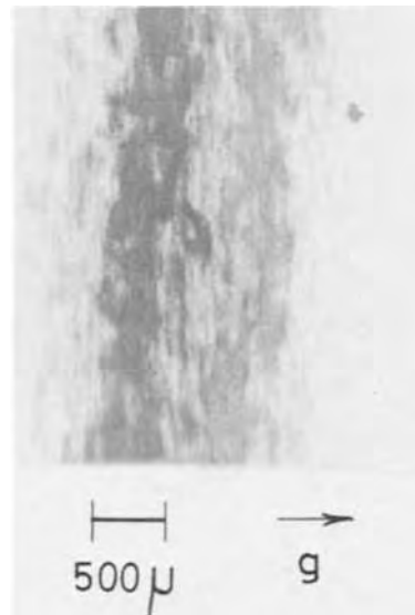
Fig. 7. X-ray topograph obtained by (220) diffraction from the GaAs 1-x P x wafer whose surface does not reveal the cross-hatch pattern.
