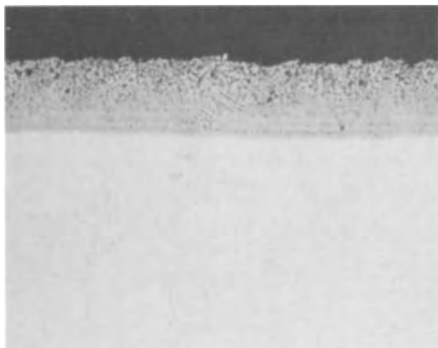
Fig. 17. Microstructure of a SermeTel J coating (190X etched)
