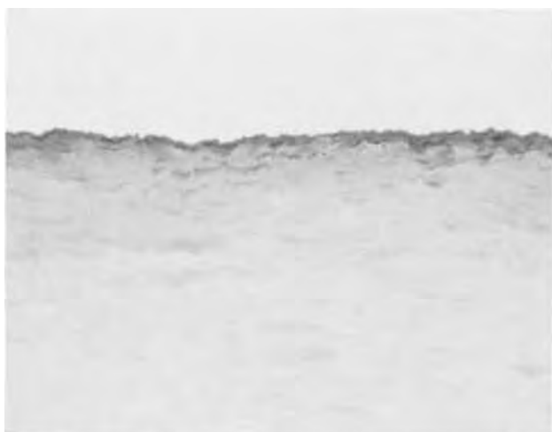
Fig. 5. Microstructure of niobium-oxide interface of niobium specimen oxidized at 430°C for 48 hr; 1400X.
