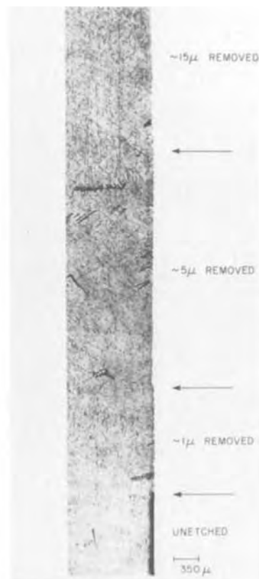
Fig. 9. X-ray topograph of a step-etched GaP wafer, diamond saw cut.
