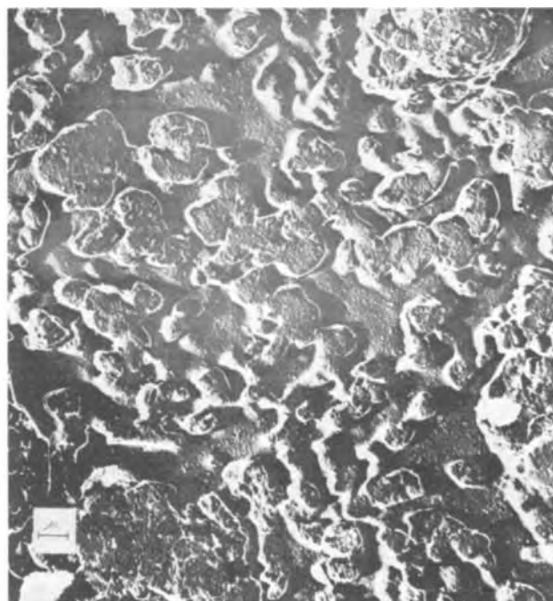
Fig. 5. Detail of tin cathode after electrolysis of TEAB/MeCN, very heavy sludging.
