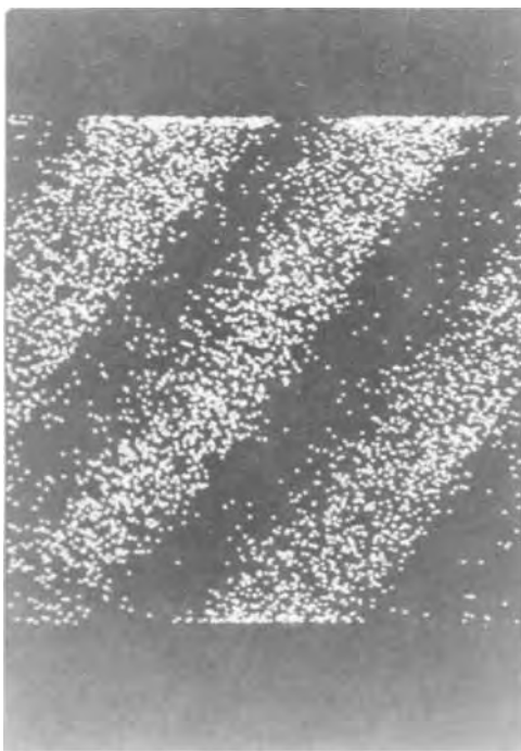
Fig. 14. X-ray image of an area of the specimen of Fig. 13, obtained with an electron microanalyzer using as signal the SbL_{\alpha} line.
