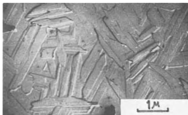
Fig. 3 (e). Carbon-platinum replica of V 2 O 5 film surface on mica, shade angle 10°.
