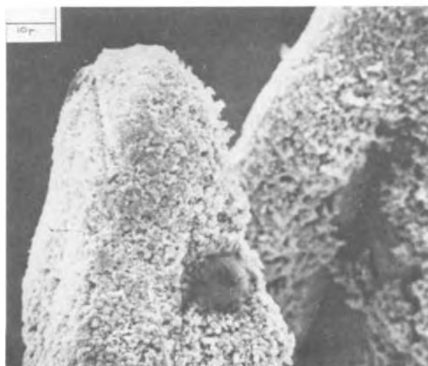
Fig. 7. Photomicrographs illustrating the dendrite tip geometry before (top) and after (bottom) solution exchange with 10^{-4}M Pb doped 10% KOH before and after solution exchange with 10^{-4}M Pb doped 10% KOH + 0.1M ZnO, \eta = -100 mV. T = 35^\circ C .
