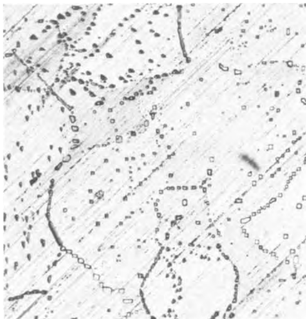
Fig. 2. Soft aluminum foil (after a 16-hr anneal at 350°C) given a 5 min dip in boiling water prior to a 550°C anneal in air. (X250).
