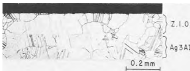
Fig. 5. Cross-section micrograph showing a zone of internal oxidation (Z.I.O.) in a Ag3Al sample which was oxidized for 29 ksec at 823°K. Etched.
