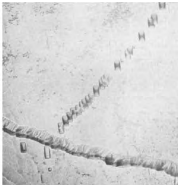
Fig. 2. Low-angle grain boundary and the pile up of dislocations against it, were revealed by HNO 3 :H 2 O (1:3), \times 350 .
