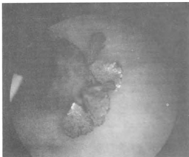
Fig. 2. Disk-type zinc morphology produced under the following conditions: 10% KOH, 0.1M ZnO, 10 -5 M Pb, \eta = -100 mV, T = 35^\circ\text{C} . Magnification X22.
