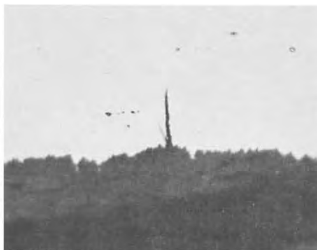
Fig. 7. Two examples showing cracks associated with niobium suboxide needles; 1400X
