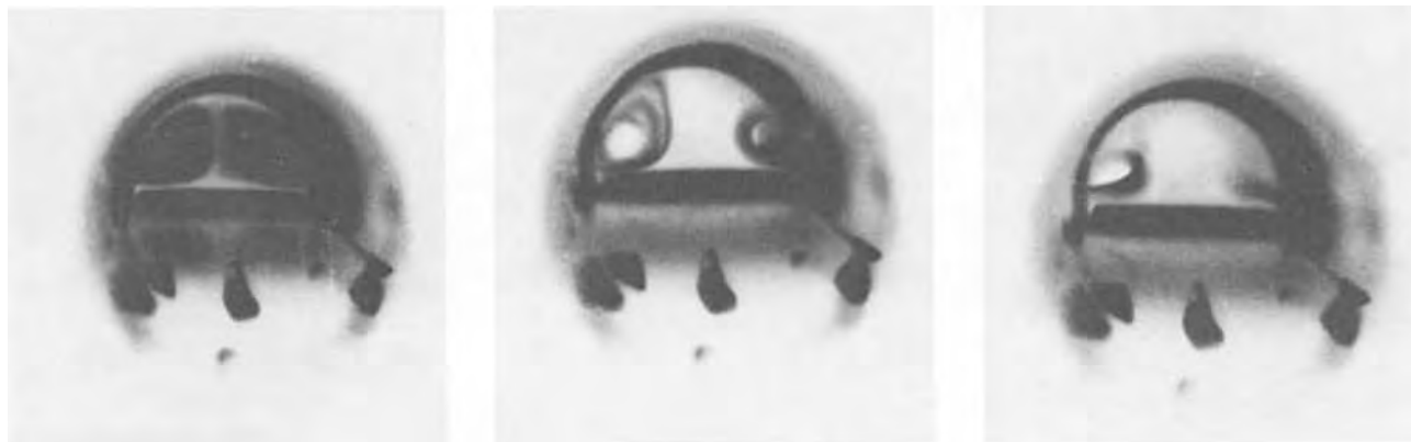
Fig. 4. Vortex patterns varying with flow rates: (a, left) He 1 liter/min; (b, center) He 5 liters/min; (c, right) He 10 liters/min
