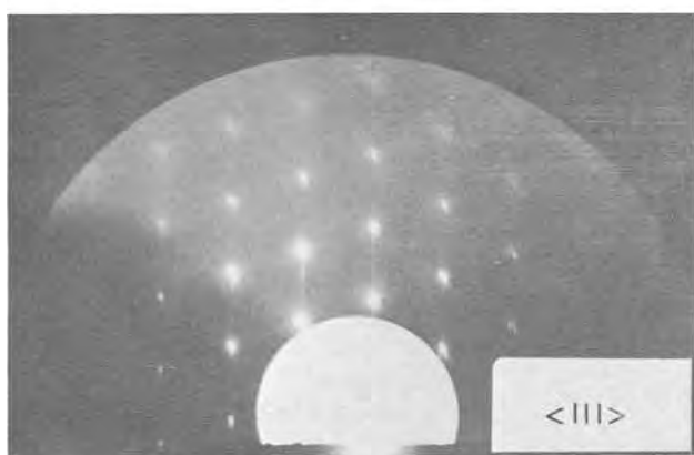
Fig. 5. (a, top) Photomicrograph, and (b, bottom) reflection electron diffraction pattern, of (111) ZnS grown epitaxially on (111) GaP on (111) GaAs.
