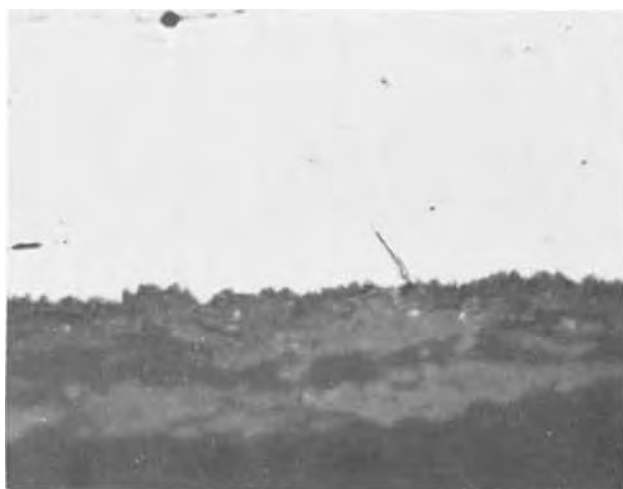
Fig. 7. Two examples showing cracks associated with niobium suboxide needles; 1400X
