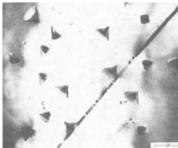
Fig. 3. Electron micrograph of substrate-annealed, oxidized copper film. The (100)-type (A), (110)-type (B), and (111)-type (C) grains are all present in this area of the oxidized film.
