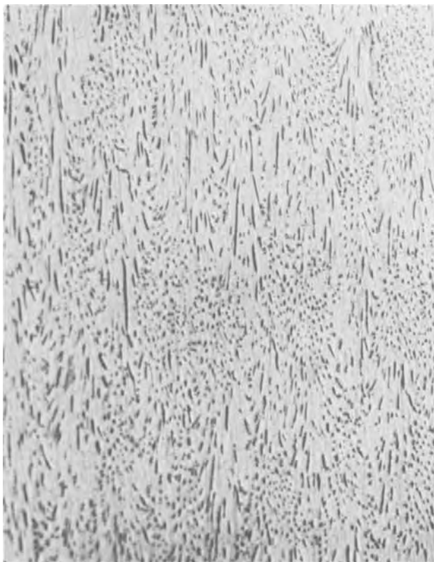
Fig. 4. Optical micrograph of bulk gold-silicon eutectic alloy. Magnification X800.
