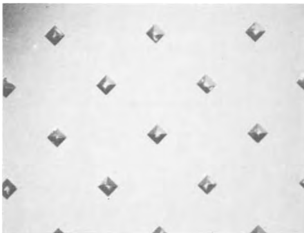
Fig. 4. Growth of undoped silicon pedestals in oxide windows on (110) substrate.
