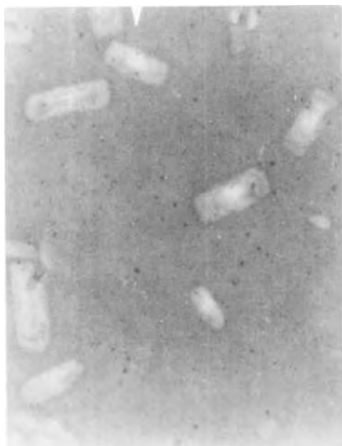
Fig. 4. Typical crystals formed by heating for a few seconds at 190°C; composition 0.6As 2 Se 3 ·0.4Sb 2 Se 3 (615X).
